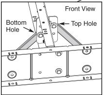
Install Cross Bars at locations shown. Secure with %" x 1½" hex bolts, %" washers and %" lock nuts.
